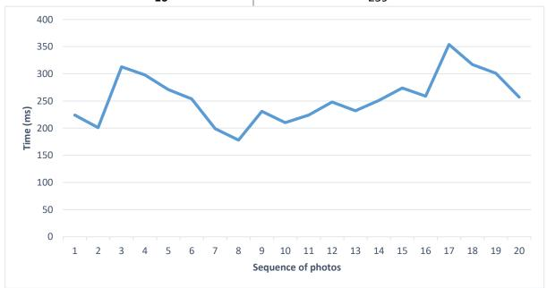
This above graph shows capture time of a photo. Checked the time with 20 photos and it gave above result which carries 64.4 ms average time for capturing one photo.
