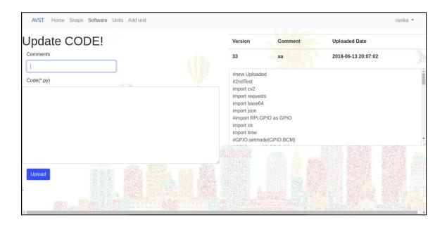
The mechanism of this system is the unit having two programs one of them is static which checkup the centralized server and update  $2^{nd}$  program if the server has a new one. The static code has unique data of unit such as ID of the unit.
