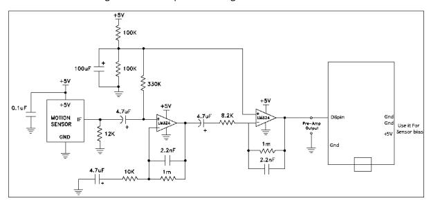
When the circuit is made up it might look like below. And the output of the circuit is connected to a raspberry pi digital pin. That pin is mentioned in python code and it measures pulse time and calculates input pulse frequency.
