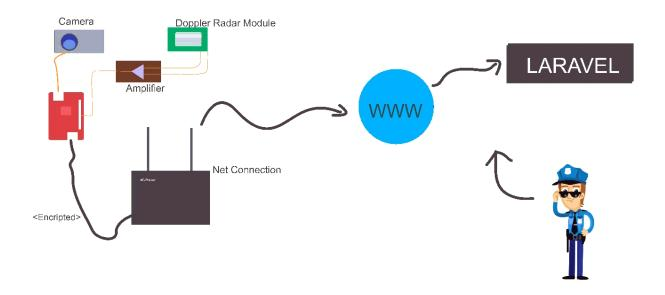
Development of the system will be placed near the expressways as below. The black box shown below will be the hardware development. It contains the sensor with the amplifier, the camera and the raspberry pi.
