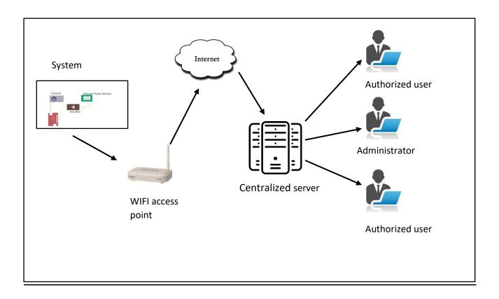
All the units are connected to one centralized server and all the data are saved in there. Data are visible to every authorized user from everywhere.
