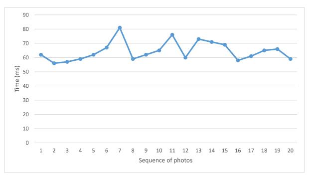
This above graph shows capture time of a photo. Checked the time with 20 photos and it gave above result which carries 64.4 ms average time for capturing one photo.
