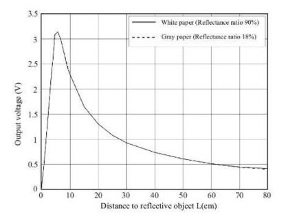
The variation of the output voltage of IR sensors against the distance to a reflective object can be modelled in the above graph. Even though the range of 0-10cm shows a gradual increase the range of 10-80cm gives us an exponential decrease.
