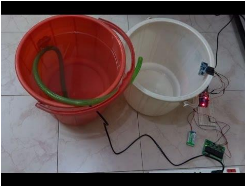
Figure 56: Apparatus to test the ultra sonic sensor
