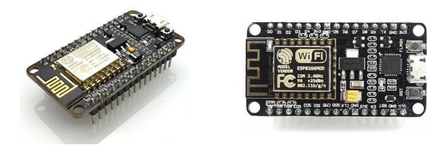
The ESP8266 is a low-cost Wi-Fi microchip with full TCP/IP stack and microcontroller capability produced by Shanghai-based Chinese manufacturer, Espressif Systems.
