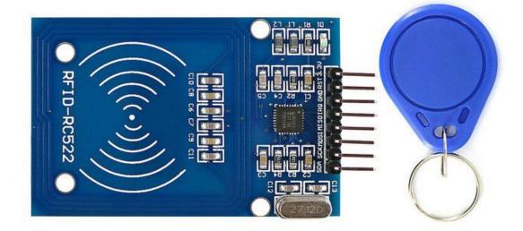
MF RC522 is a highly integrated read and write card chip applied to the 13.56MHz contactless communication. Launched by the NXP Company, it is a low-voltage, low-cost, and small-sized non-contact card chip, a best choice for intelligent instrument and portable handheld devices
