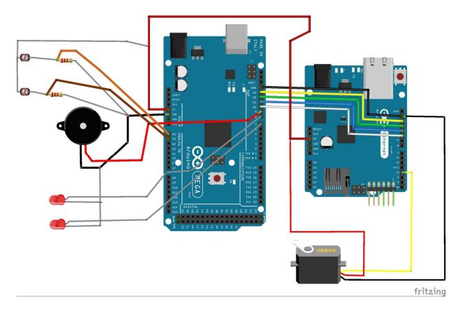
Above diagram is the gate controller of our project design. Gate controller has an arduino board, GPS module, some LDR, motor, some resistors and some wires.
