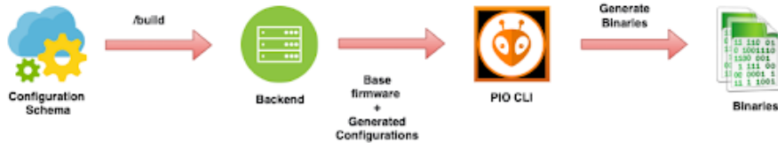
Fig. 3.3 Remote cross compiler design workflow
