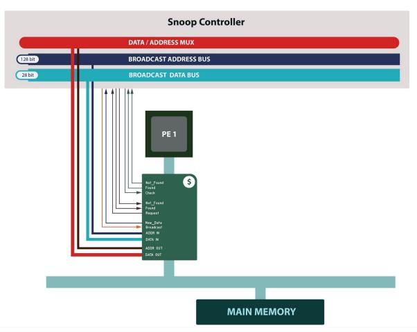
The snoop controller uses multiplexers to choose the data and address from each processing element.
