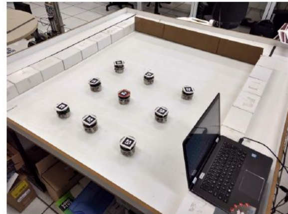
Fig. Example of a real experiment setup using nine e-pucks in two scenarios. The leader robot \mathcal{R}_l is identified by the red marker.
