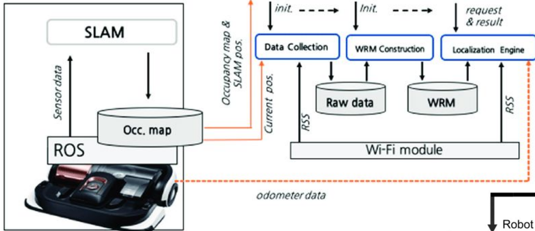
Structure of the robot localization application in SLAM system (researchgate.net)
