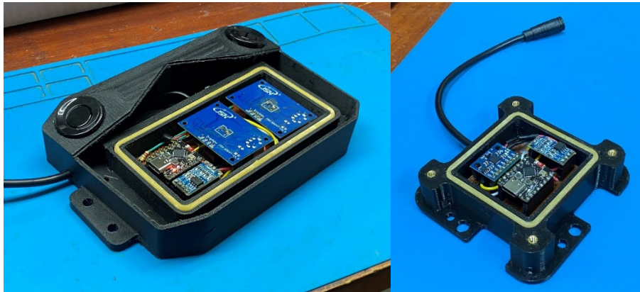
Figure 27: Rubber O-ring gaskets inside Front and Center units
