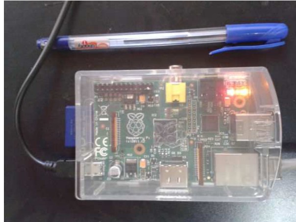
Figure 2: The Raspberry Pi miniature computer
